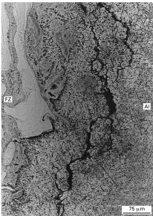
Figure 4 Cross-section of the sample welded at a speed of 1.00 \text{ m min}^{-1} and a laser power of 2.0 kW, showing intergranular crack in the resolidified zone of Al alloy: FZ, fusion zone.
