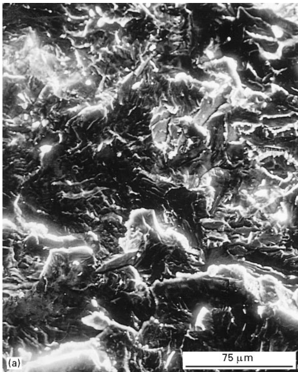
Figure 9 (a) Fractograph of the tensile test specimen without a Nb plate showing transgranular cleavage fracture. (b) Fractograph of the tensile test specimen with a Nb plate showing a large number of porosity at the interface between the Nb and the Al alloy. The inset shows a high-magnification fractograph indicating the intergranular mode of fracture.
